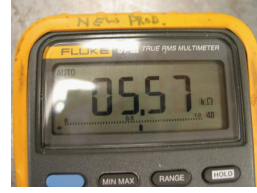
Fig. 22 – Measuring Motor NTC Resistance
